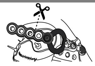
Change the screw position until you feel a slight tension when closing it (1st and 2nd holes are the most used ones). Cut the excess leaving an extra hole.
